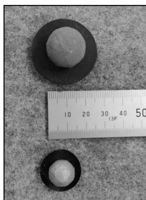
Figure 3. 3 Dimension of reflective spherical marker used
