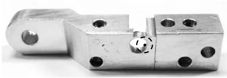
Figure 6. 6 Misaligned hole for the pin (Correct hole's position is circled in black dash)
