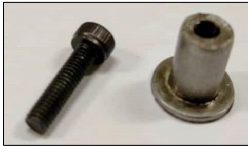
Figure 6. 4 Modified rod and 12mm length M3 screw used.
